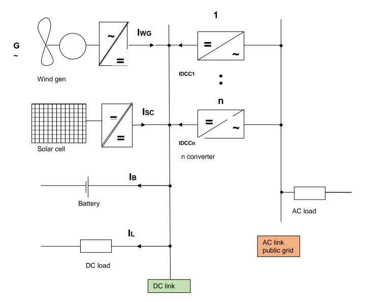
Converter keeps stable DC voltage link by controlling energy flow from AC to DC link. Converter does not have AC link control. Iwg+ Isc+ IDcc1 + ...+IDccn= IB+IL
